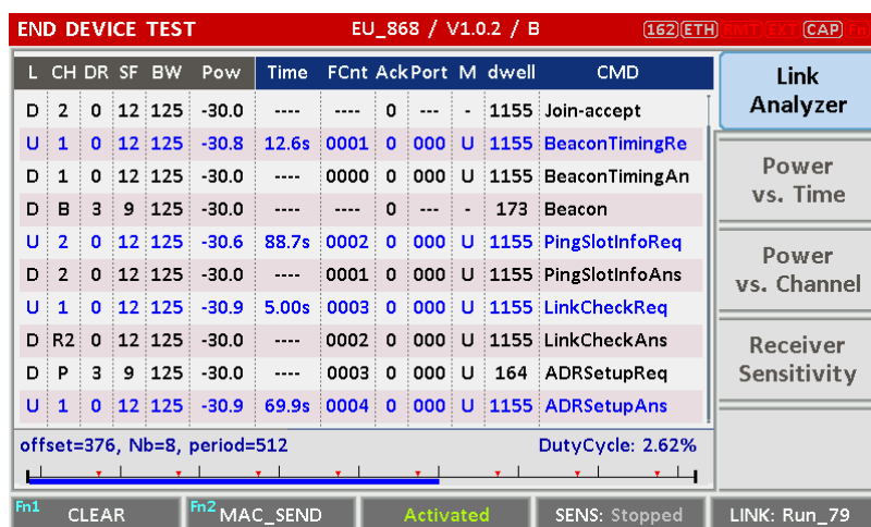
Fig 3.17 MAC command transmission through PING slot
