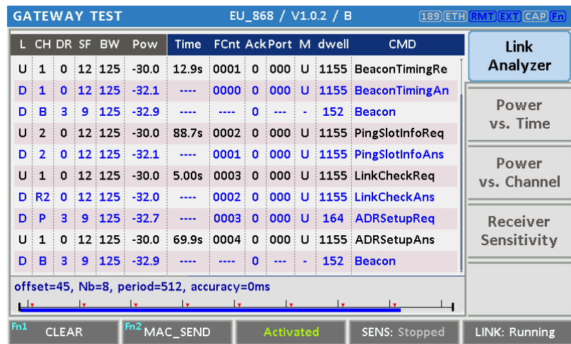
Fig 3.30 Example of communication with Class B Gateway
